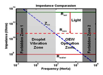
Fig. 4. Frequency response of the electrical impedance of the various components in an equivalent circuit model. OEW operation is divided into four different zones. The dashed line represents the reduced resistance of the a-Si strip under light illumination.
