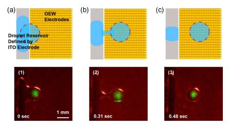
Fig. 7. Schematic diagrams and snapshots (top view) illustrating the droplet injection process. (a) Before injection. (b) In the middle of injection. (c) Injected droplet trapped by light beam.
