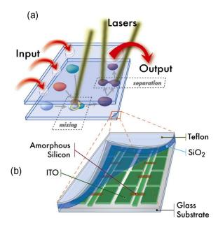
Fig. 1. (a) Schematic illustration of liquid droplet manipulation in an OEW device. (b) Schematic of the OEW device structure.
