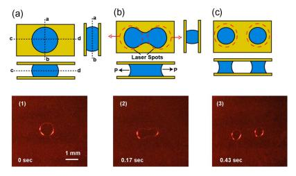
Fig. 6. Schematic drawing of the top view and two cross-sectional views (ab and cd) as well as the corresponding top-view micrographs of the droplet during separation process. (a) Before separation. (b) Two laser beams pulling the droplet along the cd direction. (c) Separation finishes.
