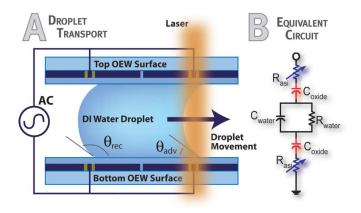
Fig. 3. (a) Illustration of contact angle change on OEW surface. (b) Equivalent circuit for one unit cell of the OEW device.  $R_{\rm asi}$  is the resistance of the a-Si photoconductor under light illumination,  $C_{\rm oxide}$  is the capacitance of the SiO<sub>2</sub> insulator, and  $C_{\rm water}$  and  $R_{\rm water}$  are the capacitance and resistance of water layer between the two OEW surfaces.
