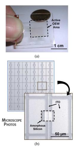
Fig. 2. (a) Fabricated OEW device (one side). The active OEW area is marked by the dashed-line square. (b) Microscopic pictures showing part of the (top) active OEW area and (bottom) structure of an OEW cell.
